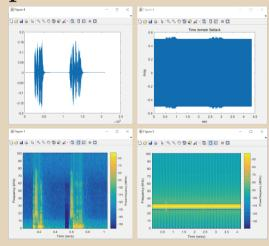
left-top: plot of original signal; left-bottom:signal spectrum diagram of origin signal; right-top: plot of attack signal; right-bottom: signal spectrum diagram of attack ignal;
